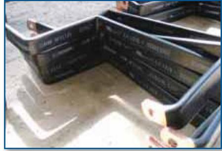
**TEKNOMEGA** makes it possible to receive Ω FLEX INSULATED FLEXIBLE BARS bent and punched as per the specific customer's requirements. This is convenient in the case of the conditions of "series" production of "standard" electric panel boards and/or equipment. The use of PREFORMED INSULATED FLEXIBLE BARS AS PER DRAWING makes it possible to optimize the wirings times and to eliminate the production of wastes and possible unused work scrap.
